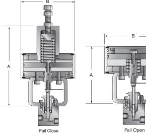
NOTE: Air inlet for Fail Close operation is located in the back, opposite the front of valve. For other locations, consult factory. Holes supplied in yoke bracket for mounting.
